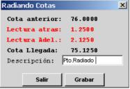
Links to databases, coordinates, banded sections, and sections type files to extract the dimensions of them to rethink. The description automatically enters information point to which belongs the elevation to rethink and obtained differences.
