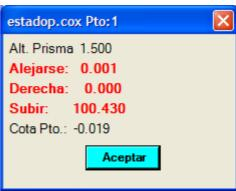
The action "Move" can be changed to "Approach" If the difference in distance is negative. The 'Right' action can be changed to "Left" and reflects the lack of alignment of the layout. "Upload" action can be changed to "Get off" depending on the difference between the real dimension and the dimension to rethink.
