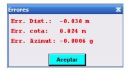
If you select only guide the program will impose an azimuth to the station, and with the third option included the previous two, i.e. focus on another base, will read it and obtain the relative errors in distance, elevation and azimuth.
