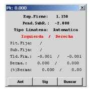
In the elements where calls are defined family of vectors are two names that are found in Pks anterior and posterior to the one requested. Interpolation vector to vector of these families will get a new set of vectors that form the figure of the type section. The slopes of the subgrade and the berms of the firm can be altered in its final application depending on the slopes of the bankings in the Pk.
