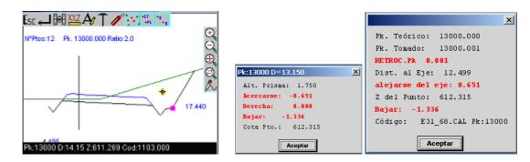
It then shows with a cross in the position of the point projected on the profile. By pressing a key displayed on screen where reports of the actual position of the point and the actions to perform for its correct position.
