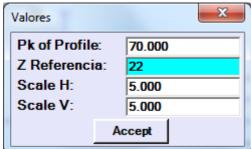
... and then shows this window where you can edit these values and also define the Horizontal and Vertical scale of the drawing in the CAD units... and finally requested to check the lines defining the work surface...
