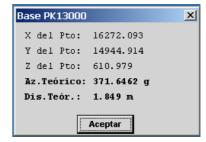
After taking the appliance reading program informs us of the location of the point taken with respect to the alignment point to rethink with the base and the actions to perform.
